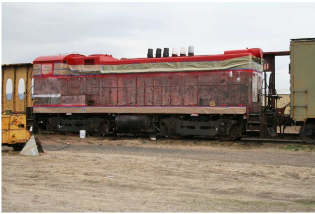
(RIGHT) This scene photographed on the afternoon of 10/30 shows No. 8 after Jerry applied the first coat of primer paint around the locomotive. It was a bit annoying to find small flying insects that were attracted to the paint and are now part of the diesel. — Tony Johnson photo
