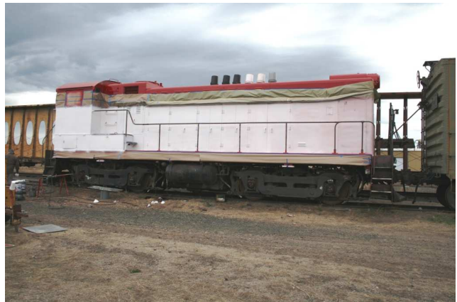
(LEFT) The 1st coat of primer is on and Art and David Turner watch Jerry mix the second coat of primer. It was mostly white in color, that is, there was a trace of the brown primer left over, creating a little marbled effect at one end. It will all be hidden under two coats of the final yellow color. — Tony Johnson photo
