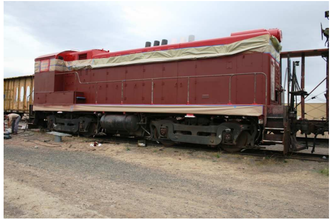
(LEFT) The 1st coat of primer is on and Art and David Turner watch Jerry mix the second coat of primer. It was mostly white in color, that is, there was a trace of the brown primer left over, creating a little marbled effect at one end. It will all be hidden under two coats of the final yellow color. — Tony Johnson photo
