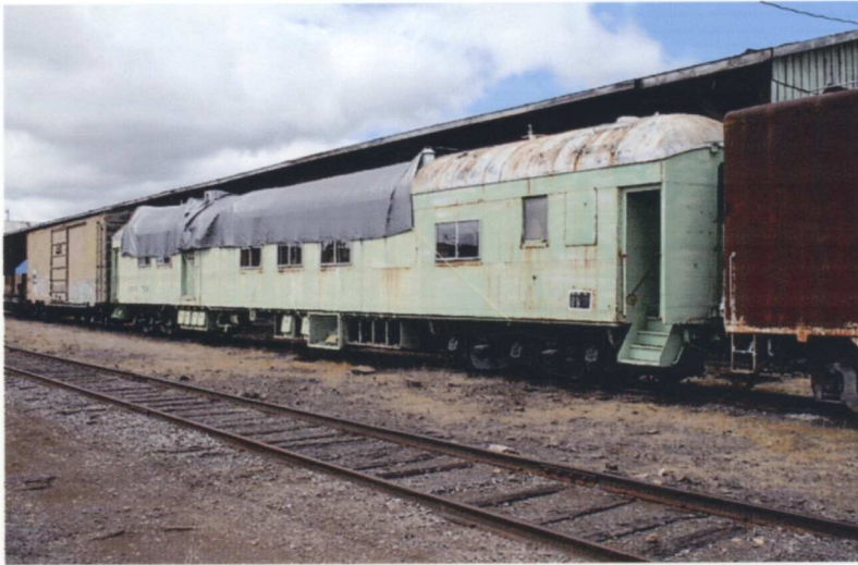
(LEFT) Our chapter's 1912 Pullman dining car is stored with other chapter equipment in White City. After transporting the car from Eugene a few years ago, we discovered leaks in the roof. As a temporary measure we protected the roof with tarps for the winter. Funding has recently been approved to patch the leaks with metal sheets and pop rivet them in place. Then we'll cover the roof with a protective fabric coating and sealant. — Tony Johnson photo
