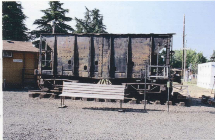
(LEFT) A few weeks after the above photo was taken, Steve Bruff began to remove the large dents around the hopper's rim. Compare a much straightened roof line against the photo above. Steve will fix the entire rim prior to painting. — Tony Johnson photo
