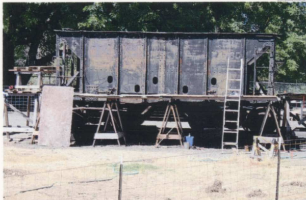
(RIGHT) Steve plans on adding another missing part. When built these cars were fitted with a wooden walkway around this side of the hopper so a worker could pound free frozen ore loose for unloading. This may be added on at a later date. — Tony Johnson photo
