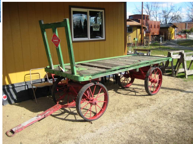
(RIGHT) This is the condition our baggage cart is in today. Since we're going to replace all the old wood, the plan is to disassemble the cart to strip the old paint off metal parts, apply new paint, and reassemble the cart. When done we'll stack several large steam trunks and boxes on the cart for a complete display. —Rick Aubin photo
