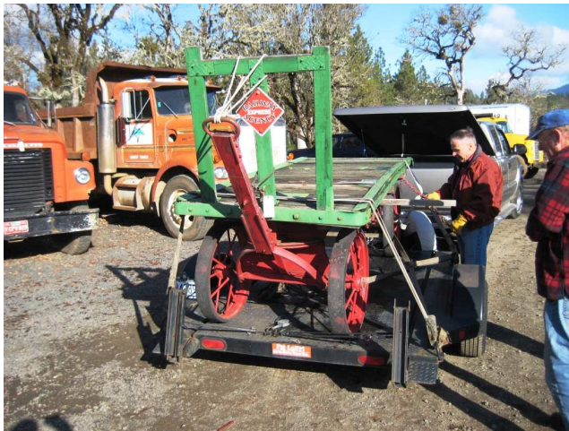
(RIGHT) This is the condition our baggage cart is in today. Since we're going to replace all the old wood, the plan is to disassemble the cart to strip the old paint off metal parts, apply new paint, and reassemble the cart. When done we'll stack several large steam trunks and boxes on the cart for a complete display. —Rick Aubin photo
