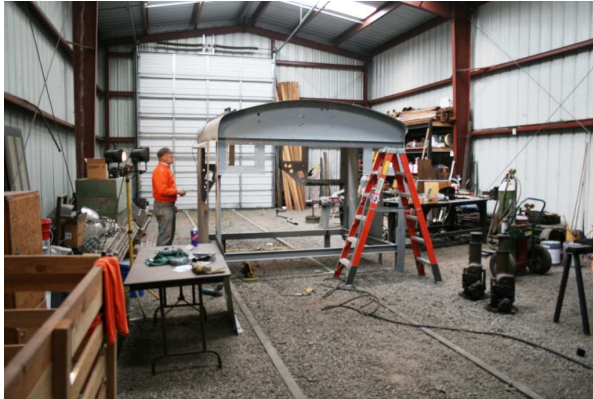
[ABOVE] Last month we showed you a photo of the cab of Medco No. 4 after being cleaned by shot blasting and finished with a coat of primer paint. These images were taken after moving the locomotive outside and the cab inside. Before painting Jerry prepared any areas still needing preparation; followed by painting the metal black with Zero Rust paint. — Tony Johnson photos
