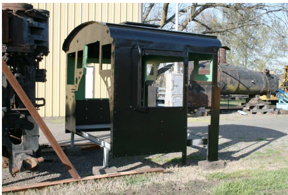
[ABOVE, LEFT] This view shows the fireman's side of the cab after painting. The next step for the cab will be to cut and shape new wood to line the cab's interior. [ABOVE, RIGHT] Visitors to the Railroad Park this season will be able to see the frame, trucks, oil tank, water tank and other parts from outside the engine house. We realize that many past park visitors never bothered to look to see if there was anything inside the engine house. Now our locomotive will be out in the open. — Tony Johnson
