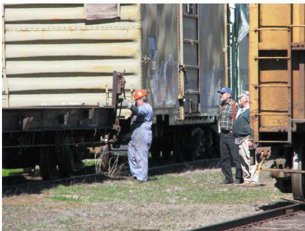
[ABOVE, LEFT] Jerry Hellinga and Art Turner watch as the WCTU conductor releases hand brakes on all three cars to be moved. [ABOVE, RIGHT] All three cars are now clear from their former storage track and are ready to be shoved into the spur with the protective roof. Here you can see the numerous blue tarps we used to protect the leaky roof from further rain damage. The boxcar will be used to store supplies and tools. — Roger Phillips photos
