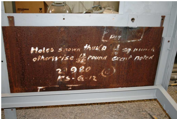
[ABOVE, LEFT] Prior to shot blasting and painting, any original specs painted by the builder back in 1925 were covered over for preservation. They are still there and will be covered when we install new wood lining in the cab. [ABOVE, RIGHT] Here is the engineer's side of the cab after painting. The interior is now painted green, just like it was when it left the builder. — Tony Johnson photos
