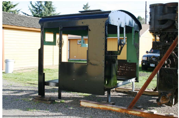
[ABOVE, LEFT] Prior to shot blasting and painting, any original specs painted by the builder back in 1925 were covered over for preservation. They are still there and will be covered when we install new wood lining in the cab. [ABOVE, RIGHT] Here is the engineer's side of the cab after painting. The interior is now painted green, just like it was when it left the builder. — Tony Johnson photos
