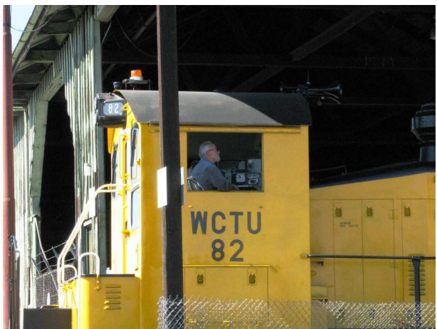
[ABOVE, LEFT] The engineer slowly advances the cars forward to the new location. WCTU #82 is a model SW1200 built by EMD in 1965 for the Richmond, Fredericksburg & Potomac in 1965. WCTU Railway acquired the locomotive in 2001. [ABOVE, RIGHT] Easy does it. Our three cars are carefully positioned to where we will work on repairing the roof of the dining car. It's a blessing for us to have this location. — Roger Phillips photos
