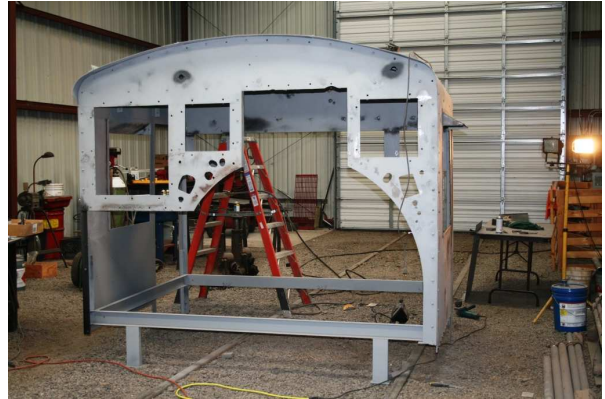
[ABOVE] Last month we showed you a photo of the cab of Medco No. 4 after being cleaned by shot blasting and finished with a coat of primer paint. These images were taken after moving the locomotive outside and the cab inside. Before painting Jerry prepared any areas still needing preparation; followed by painting the metal black with Zero Rust paint. — Tony Johnson photos
