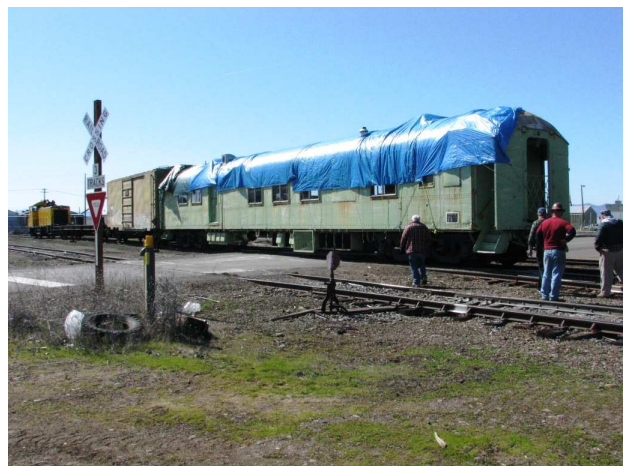
[ABOVE, LEFT] Jerry Hellinga and Art Turner watch as the WCTU conductor releases hand brakes on all three cars to be moved. [ABOVE, RIGHT] All three cars are now clear from their former storage track and are ready to be shoved into the spur with the protective roof. Here you can see the numerous blue tarps we used to protect the leaky roof from further rain damage. The boxcar will be used to store supplies and tools. — Roger Phillips photos
