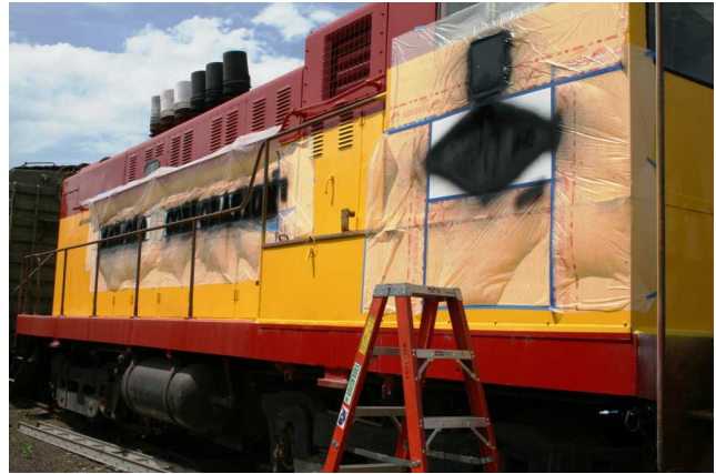
[LEFT] Joe Berto carefully measures exactly where each letter of the vinyl stencil is to be located on the hood. After removing the each letter, butcher-type paper is taped around the area to protect the hood’s yellow paint. — Tony Johnson photo
