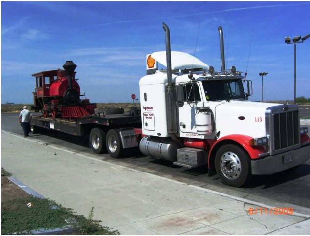
[RIGHT] RRV #1 wasn't just a static display on top of a lowboy trailer. The engine crew actually operated the boiler under steam pressure so the whistle could operate during and after the town's celebration parade. The Jacksonville Fire Department supplied the water for the locomotive via one of their pumper trucks. — Ric Aubin photo
