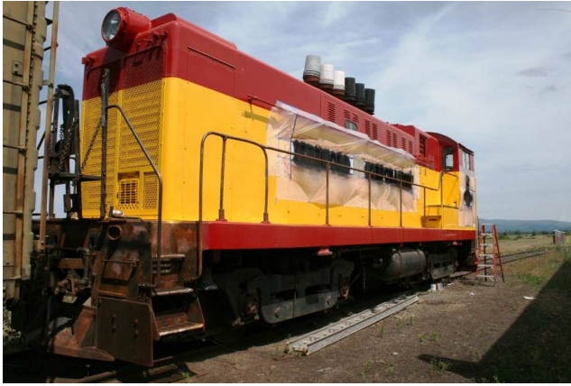
[LEFT] Another step towards returning Medco No. 8 back to her original appearance came when Jerry Hellinga and Joseph Berto took a few days to apply “Medford Corporation” to the long hood, and the famous MEDCO diamond logo and number to the cab. This view of the fireman’s side shows the black paint already has been applied over the stencils and protective paper. — Tony Johnson photo
