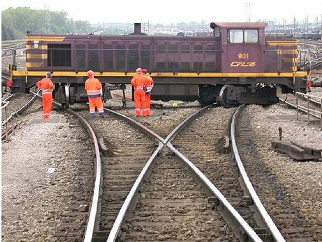
It is not good to thro a switch in the middle of a locomotive.
