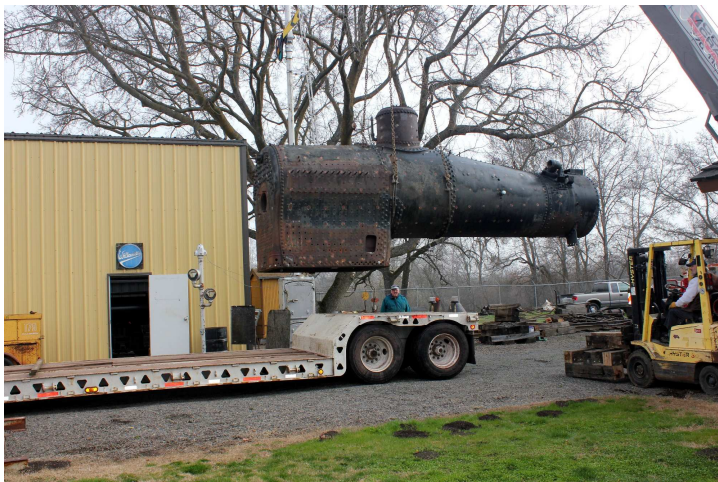
The trailer is being moved under a floating boiler.
